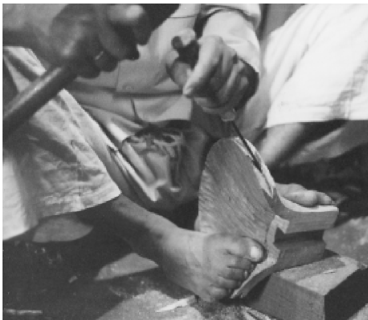
The shaping of the gulu is accomplished two stages after the rough shape has seasoned for at least 6 months. This shows Hari chiseling the rabbit in the gulu that will receive the tumba. Typical of Step 4
