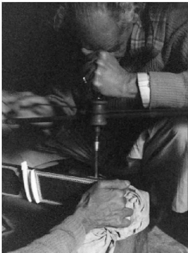
Drilling for the first five tuning pegs using the bow-drill.
