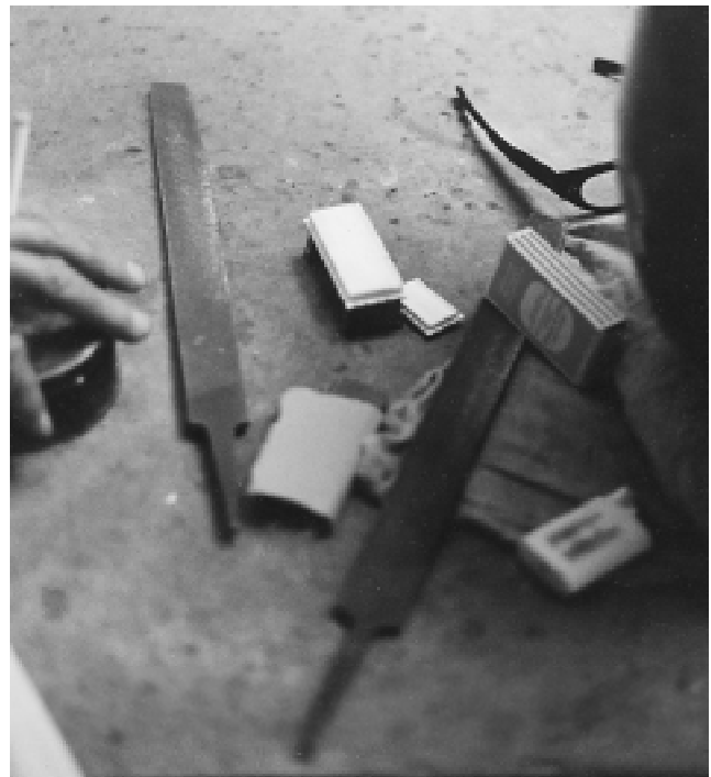
Tools for 'doing the jiwari ': Coarse and medium double-cut files, sanding block with 100x sandpaper, pack of smokes.
